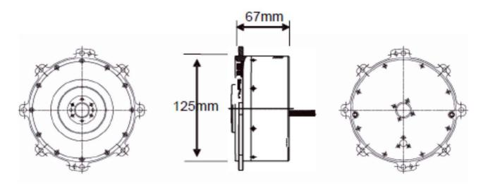
(Note) The above figure of 125 mm corresponds to the outer diameter of the case not including the attachment flange. The actual attachment flange will be coordinated case by case.
